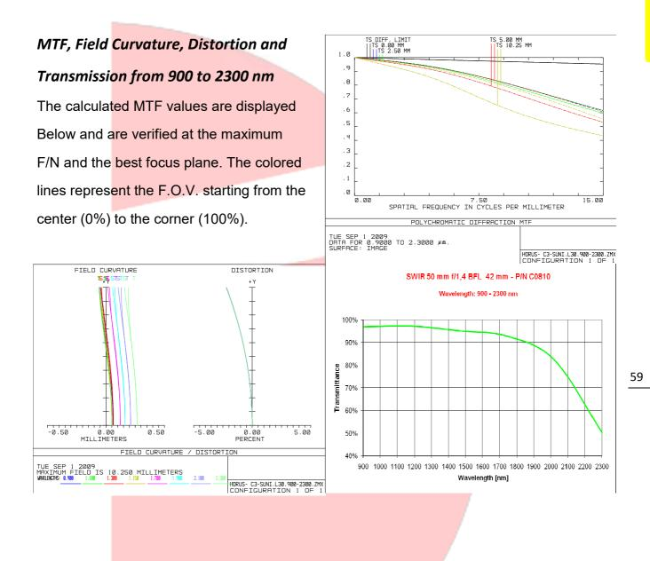
Optical parameters for wavelength range 0.9 – 2.3  $\mu m$
