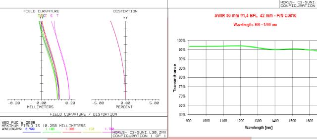
Optical parameters for wavelength range 0.9 – 1.7  $\mu m$
